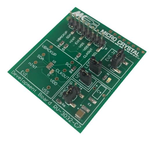
Temperature Sensor & RTC Module
