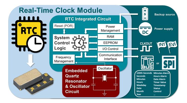
By assembling the Quartz Crystal and the Real-Time Clock integrated circuit within a single RTC package, Micro Crystal's RTCs allow to minimize the footprint. It does not require any oscillator adjustment during OEM's design phase, minimizing integration constraints thus lowering development cost and time to market. The factory calibration process and the hermetic package ensure high accuracy and stability over lifetime thus high reliability of these devices.
