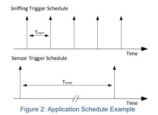
According to typical low-power application needs, it can be considered that the sensor measurements are performed at a periodicity ( $T_{SENSE}$ ) larger than one minute and can even be defined in hours or days. In contrast, the sniffing period ( $T_{SNIFF}$ ) is expected to be in the range of seconds in order to detect the request for communication sent by the base station collecting measurement data.
