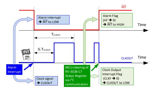
Figure 7: Alarm Interrupt active and clearing operation
