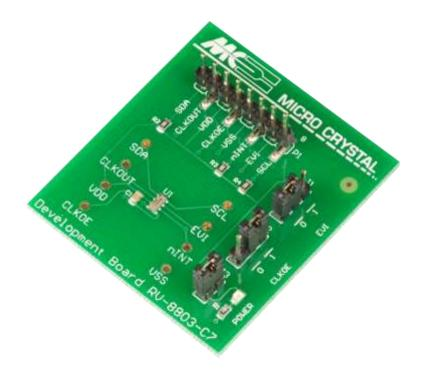
Temperature Compensated Real Time Clock / Calendar Module
