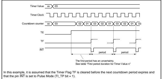
If a new Timer Value is written before the end of the current timer period, then this value takes immediate effect. It is not recommended changing the Timer Value without first disabling the counter by setting bit TE logic 0. The update of the Timer Value is asynchronous to the Timer Clock.
