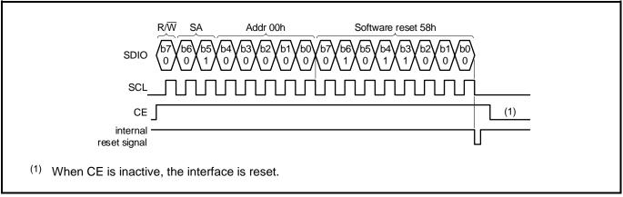
In reset state all registers are set according to the Table in section REGISTER RESET VALUES SUMMARY and the address pointer points to no address.
