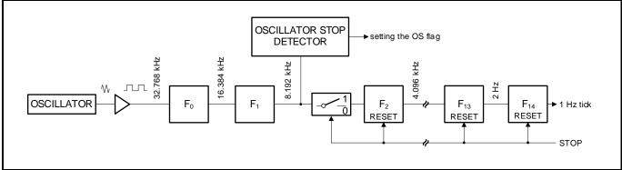
The time circuits can then be set and do not increment until the STOP bit is released (see following Table and Figure).
