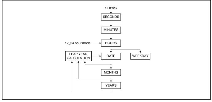
During read/write operations, the time counting registers (memory locations 04h through 0Ah) are frozen for 1 second.
