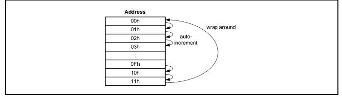
All registers (see REGISTER OVERVIEW) are designed as addressable 8-bit parallel registers although not all bits are implemented.
