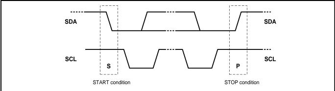
Both SDA data and SCL clock lines remain HIGH when the bus is not busy.
