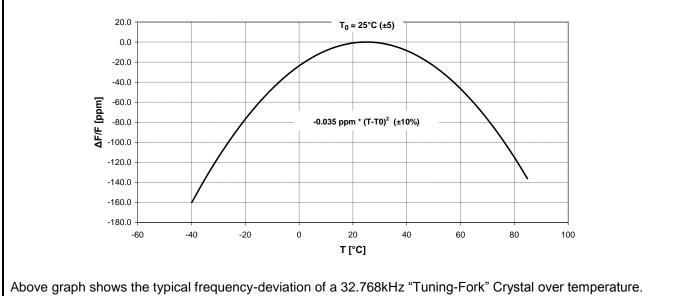
Above graph shows the typical frequency-deviation of a 32.768kHz "Tuning-Fork" Crystal over temperature. The parabolic curve is specified in terms of turnover temperature " $T_0$ " and the quadratic thermal coefficient " $\beta$ ".
