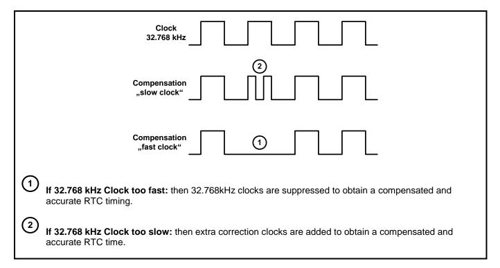
Each compensation period takes 32 seconds. Correction clocks are periodically applied during one complete compensation period. Within a compensation period of 32 seconds, one correction clock will compensate the time information by  $\pm 1$  ppm.
